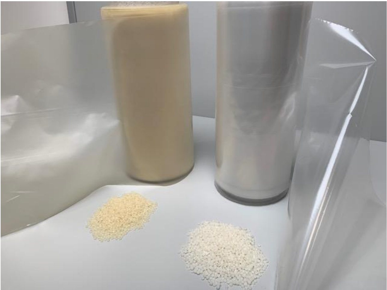
In the picture above: on the left granules obtained by regrinding laminated film with glue and re-extruded film. On the right, granules obtained by regrinding a thermal laminated PE/PE and re-extruded film.
